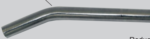
Bowed pipe No. 3a/DN 40
