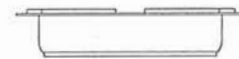
RECESSED AIR GAP When spherical or hard to hold iron is present
